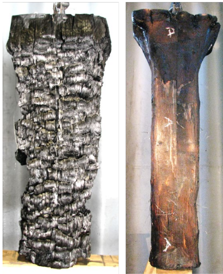
Figure 3: Glulam column after 180-minute exposure to the standard fire (left) and with the char layer removed (right).
