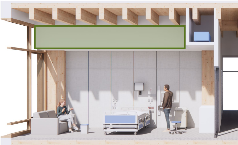
OPTION B BUILT-UP ASSEMBLY • Exposed CLT ceiling • 1,055 SF of 1" acoustic wall panel (NRC 0.8) at upper walls
